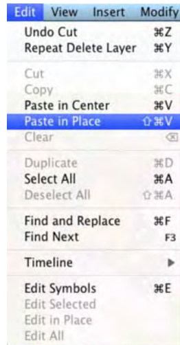
Figure 1-36. Paste in Place pastes objects in the precise location of the original object that was either cut or copied to the clipboard.
